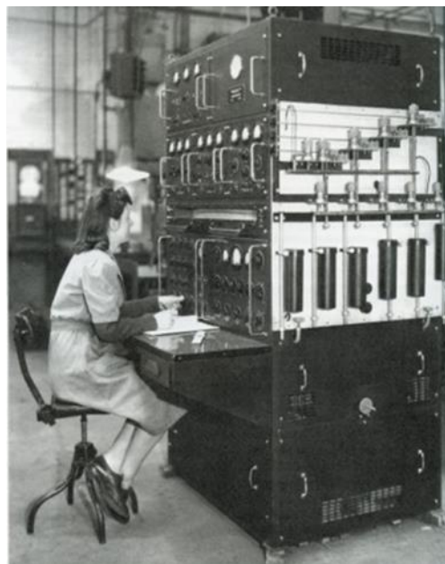
MS1 (1946): Analysis of isotope ratios in uranium hexafluoride (UF 6 ) contained in gas cylinders on the side of the instrument by mathematician Anne Mettrick from MV. This is likely to be the fourth MS1 which remained at MV and was used to develop MS2.
