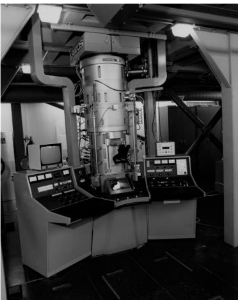
AEI/Kratos 1 MV transmission electron microscope console.
